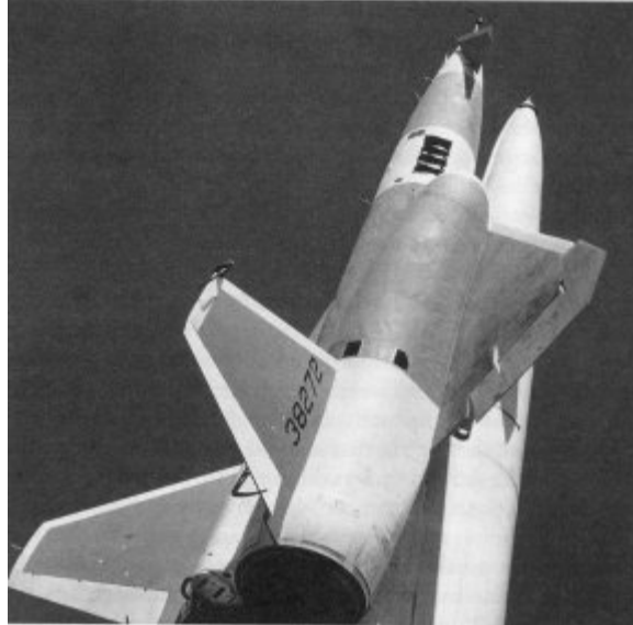
Photo from the James Gil/son Collection G-26 Vehicle No.5 (8272) in close-up on the pad at Complex Nine. The metal hook on the rudder measured control surface deflection. Note that the covers are not on the instrument compartment. The structural rings give the appearance of being vents.
