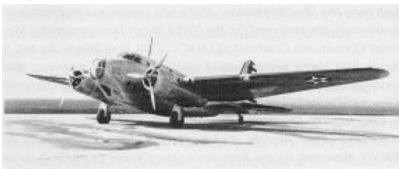
Photo courtesy of the Boeing History Archives Office The NA-21 with supercharger ducting relocated to the through sides of the engines and the actual turrets installed became the NA-39 and was designated the XB-21.
